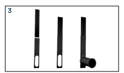
Extend the adjustable window slide kit to the length of your window and secure with the wing nut supplied. Connect the exhaust hose to the window kit.
