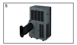
Attach the hose connector to the exhaust air outlet of the unit.
